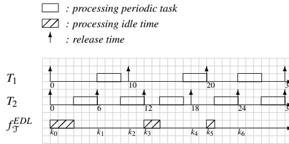
Figure 3:  $f_{\mathcal{J}}^{EDL}$  computation produced at time zero
