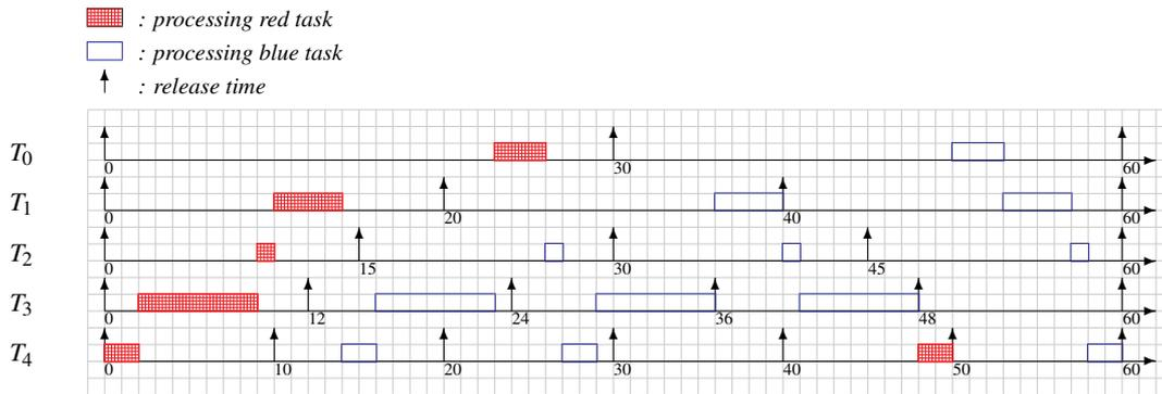
Figure 5: RLP/T scheduling algorithm ( $s_i = 2$ )
