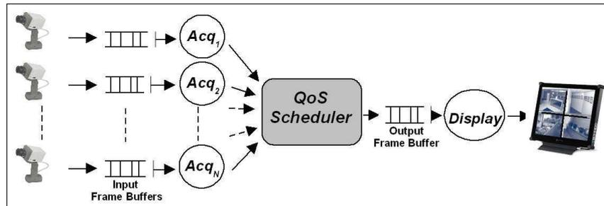
Figure 6: Simplified architecture of a real-time telesurveillance application
