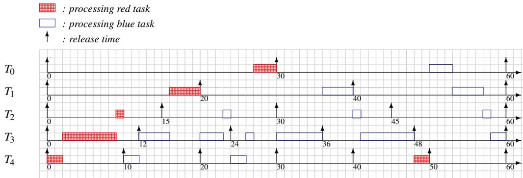
Figure 4: RLP scheduling algorithm ( $s_i = 2$ )
